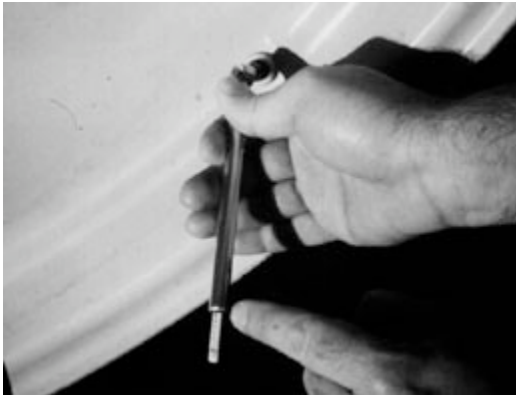
Figure 3. Checking for proper pressure.
