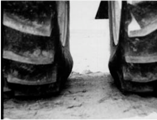
Figure 2. Properly inflated radials should have a sidewall "cheek" or bulge.
